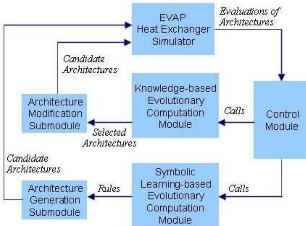
Figure 2. A functional architecture of ISHED1.
