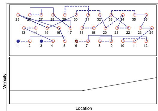
Figure 6. ISHED1-generated refrigerant circuitry for non-uniform air distribution:
