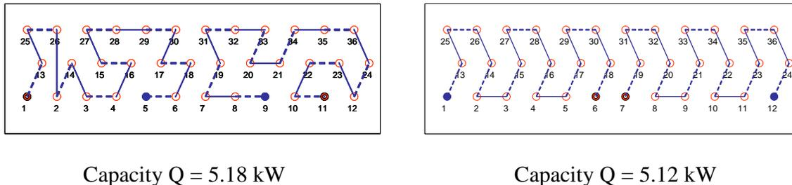
Figure 5. Two modified circuitry designs for uniform air distribution
