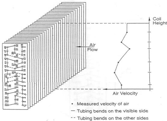
heat exchanger strongly depends on the order in which the tubes are connected.
