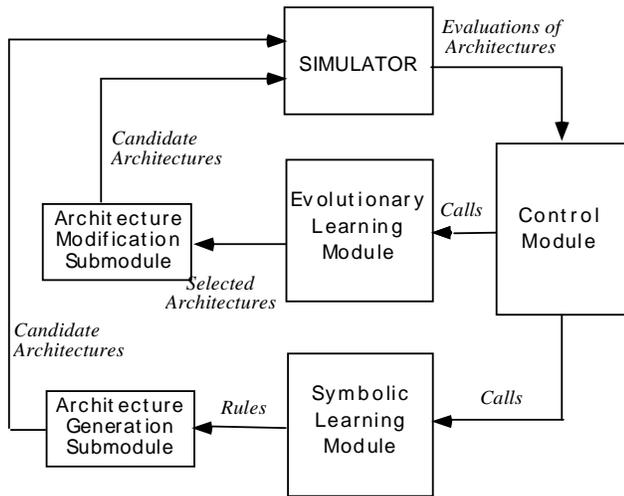
Figure 2: A general functional architecture of ISHED1.
